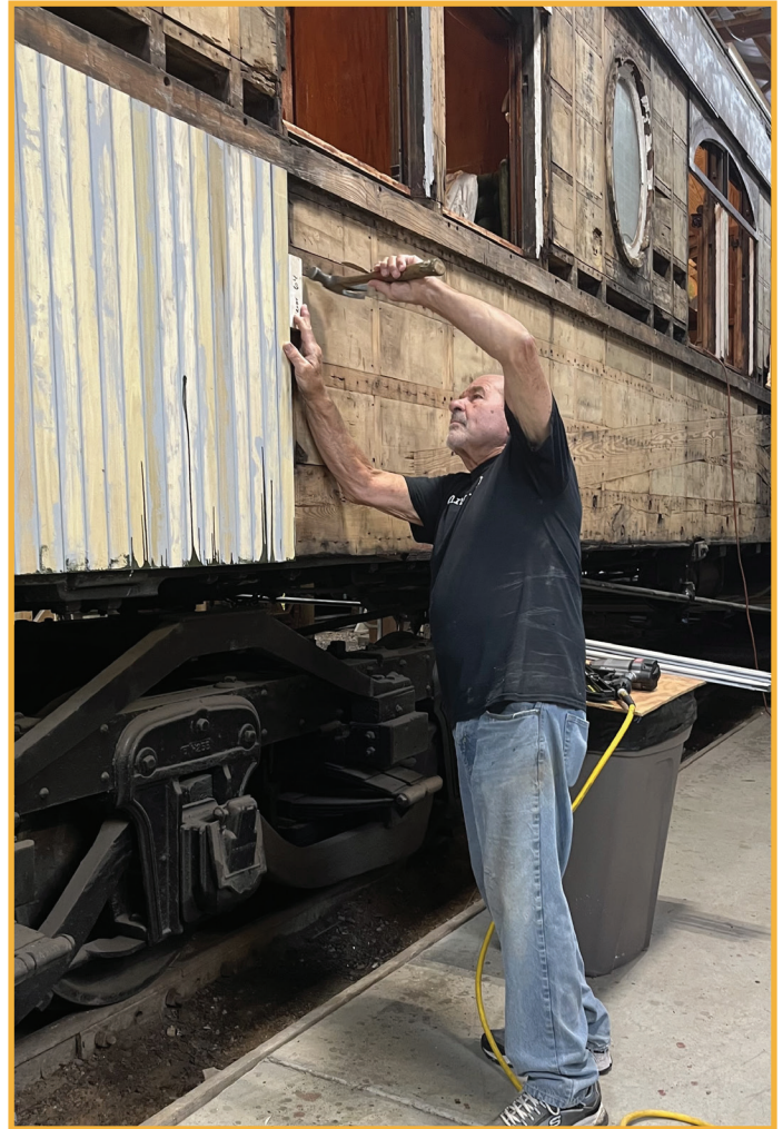
Volunteers in the process of installing new car siding on the lower portion of the car (R and L). A portion of the replacement belt rail sill is visible above the new siding (L).
