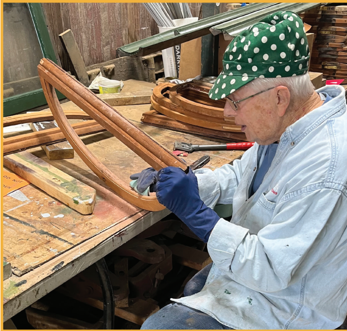
Stripping and sanding in process on one of the single light clerestory windows (L) and hand lettering the numbers on the berth headboards (R).
