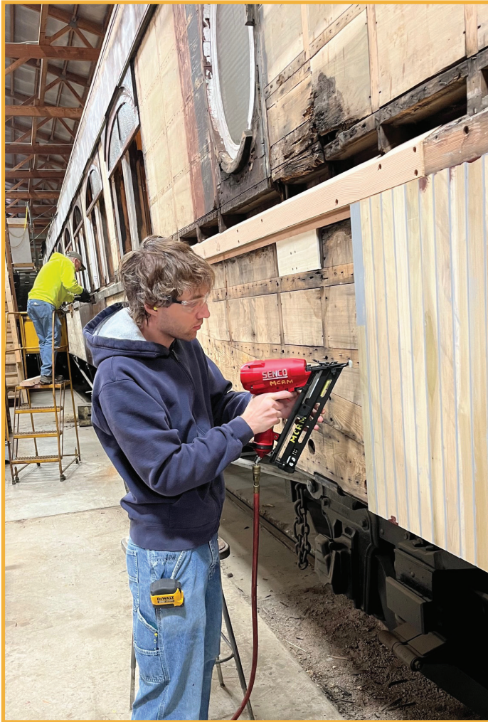
Volunteers in the process of installing new car siding on the lower portion of the car (R and L). A portion of the replacement belt rail sill is visible above the new siding (L).
