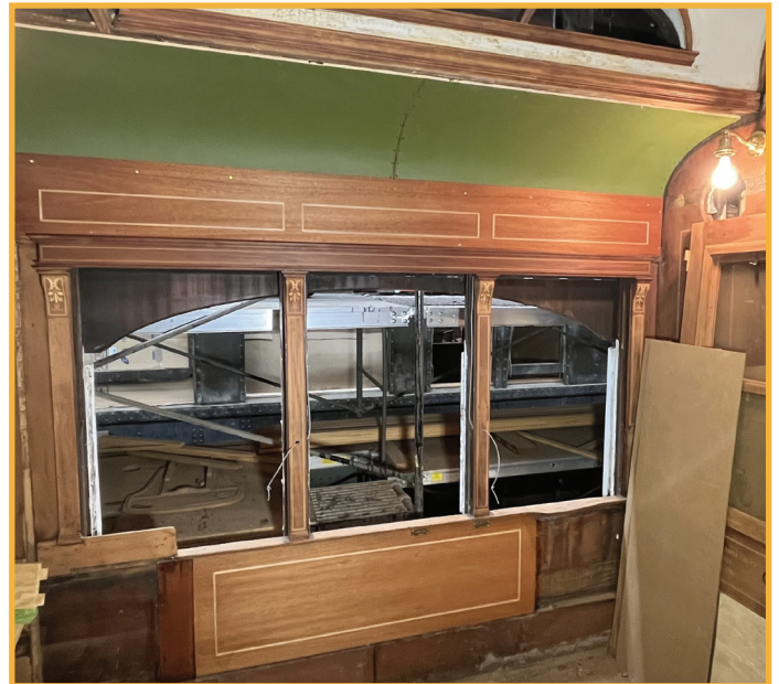
Installing trim around the new headliner in the aisle across from the smoking room (L). The smoking room outer wall with the replicated veneer in place and the new headliners (R).
