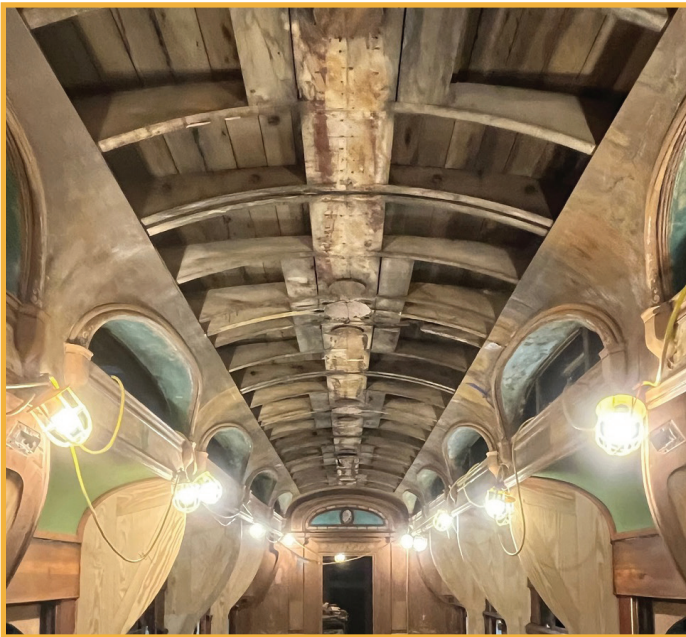
The ceiling area awaiting replacement (L) and volunteers installing the new bending plywood material (R).
