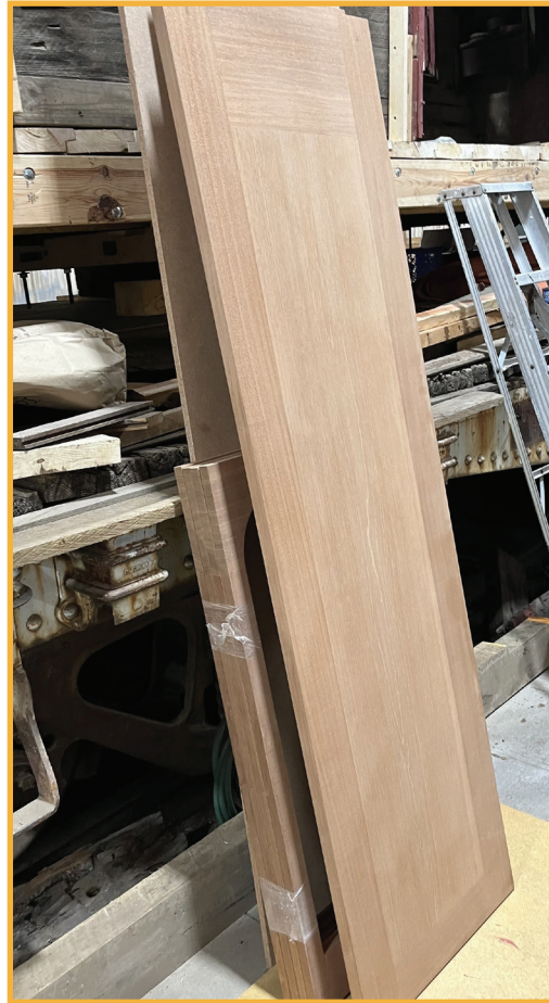
Three new interior doors and four new vestibule window frames (behind the door) replicated for the car.
