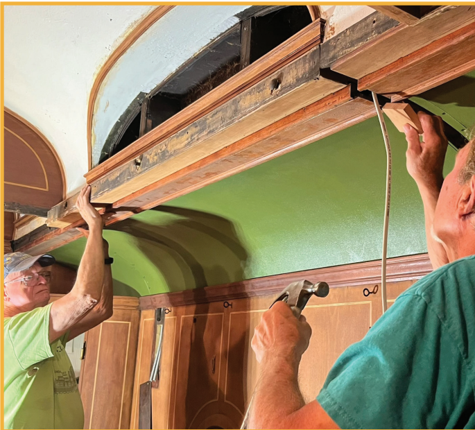
Installing trim around the new headliner in the aisle across from the smoking room (L). The smoking room outer wall with the replicated veneer in place and the new headliners (R).
