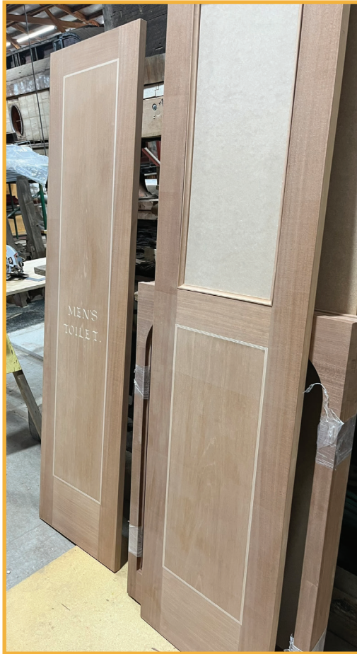
Three new interior doors and four new vestibule window frames (behind the door) replicated for the car.
