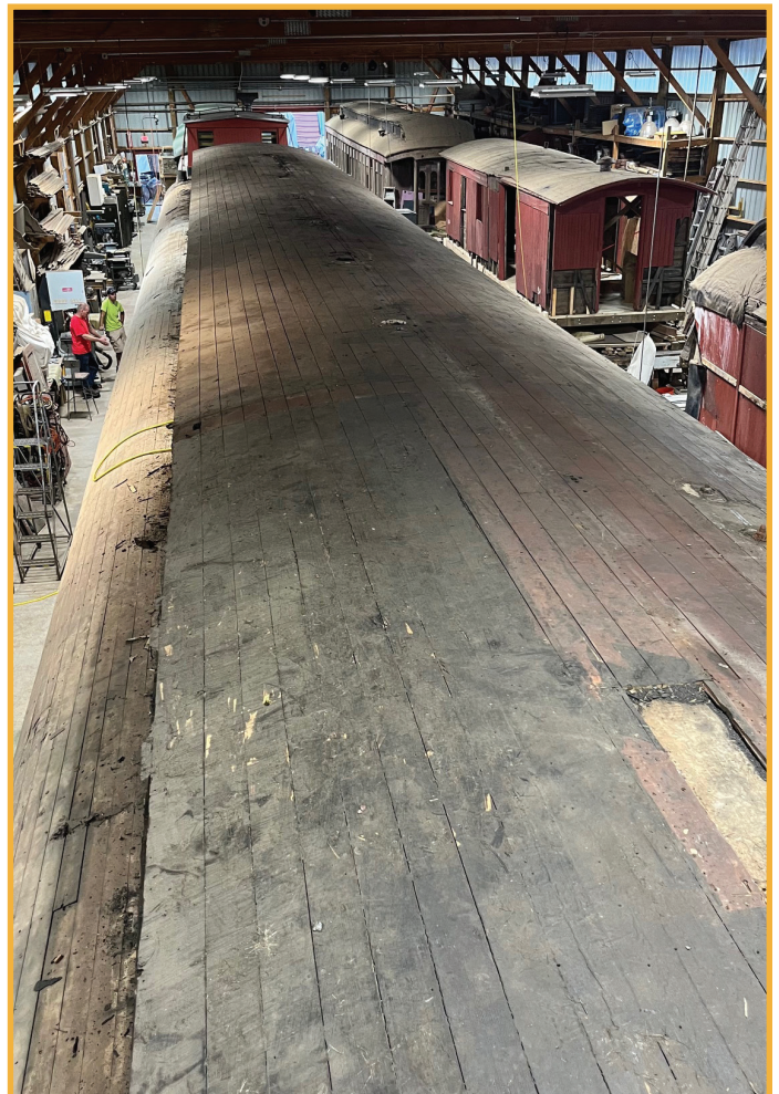
Volunteers in the process of removing the electrical wiring, etc. off the upper roof (L) and after everything was removed (R).
